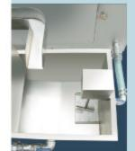
YC Mechanism Brine Injector ZSI-140 is designed stainless steel with the function to adjust the stepping speed and stroke as per the specific product and process requirements, so as to evenly inject the saline and the pickle agent into the meat slices and bone-borne meat, giving a shorter pickling period.
