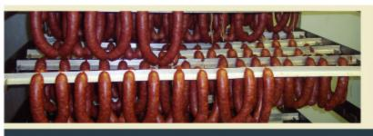
YC Mechanism Smokehouse is completely constructed of stainless steel and can be easily cleaned. The standard smokehouse, air is circulated 14 times per minute with a specially design circulating fan. A specially designed mixing chamber enables you to combine low temperature and high temperature air, smoke and low pressure steam so that the product in the smokehouse can be perfectly processed. Ensures a uniformly cooked product with constant core temperatures and
